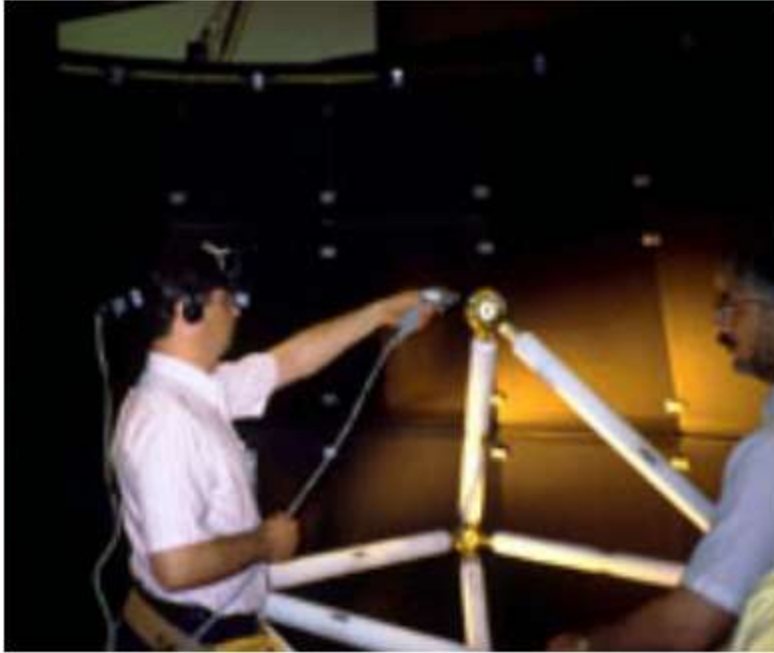
F. AR applied to Engineering Design. This figure shows a real object augmented with virtual tubes[18].
